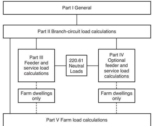
**Figure 220.1 Branch-Circuit, Feeder, and Service Calculation Methods.**
