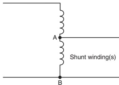
**Figure 450.4 Autotransformer.**
