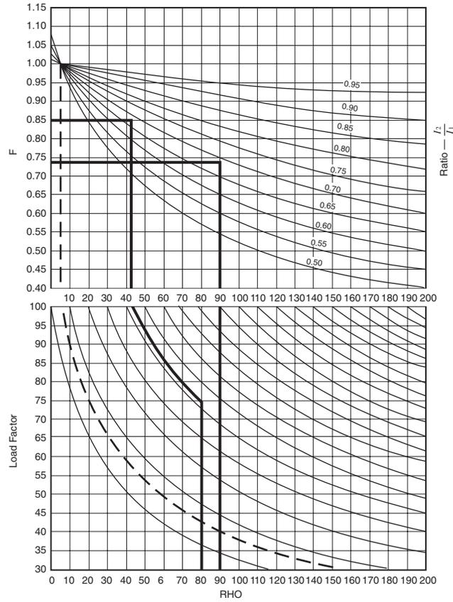
**Figure B.310.15(B)(2)(1) Interpolation Chart for Cables in a Duct Bank  $I_1$  = ampacity for Rho = 60, 50 LF;  $I_2$  = ampacity for Rho = 120, 100 LF ( load factor); desired ampacity =  $F \times I_1$ .**
