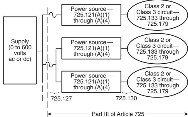
Figure 725.121 Class 2 and Class 3 Circuits.
