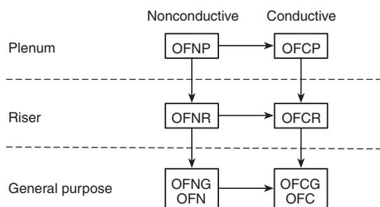
**A** → **B** Cable A shall be permitted to be used in place of Cable B.
