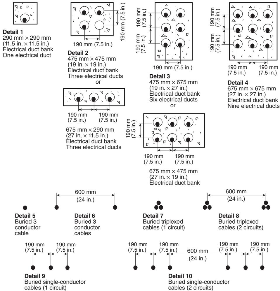
Note 1: Minimum burial depths to top electrical ducts or cables shall be in accordance with 300.5. Maximum depth to the top of electrical duct banks shall be 750 mm (30 in.) and maximum depth to the top of direct buried cables shall be 900 mm (36 in.)
