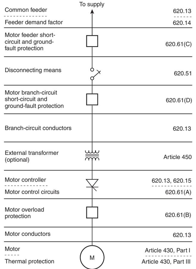
**Figure 620.13 Single-Line Diagram.**
