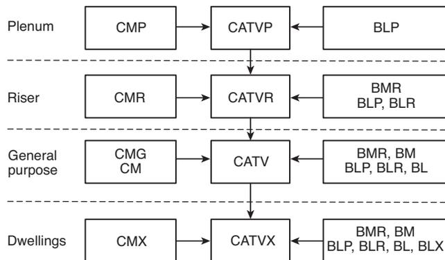
**[A] → [B]** Coaxial cable A shall be permitted to be used in place of coaxial cable B.
